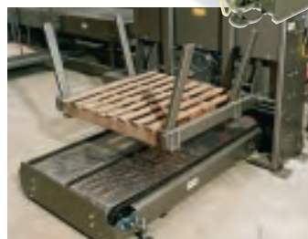
Our optional automatic pallet stacker enables the bulk container depalletizer to operate with minimal operator attention.
