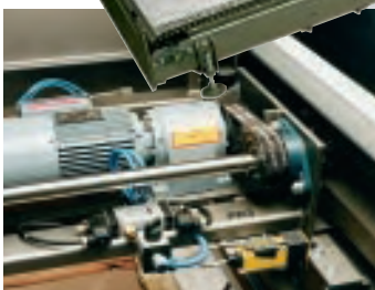
Priority One® uses timing belts to reduce wear, backlash and tensioning found with comparable chain drive systems.
