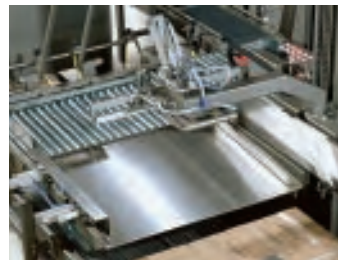
Priority One's Pro-Pal ® Mini stripper bar with landing gear, for handling small cases and shrink wrapped trays.
