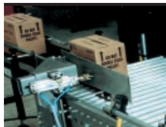
A pre-programmed control determines which cases need to be turned or deflected for pattern formation.
