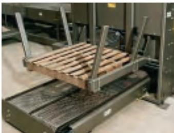
The pallet dispenser feeds empty pallets to the system automatically.
