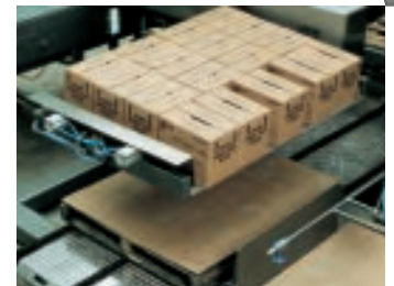
Layers are transferred to the load one at a time... minimizing wear and tear on the system.
